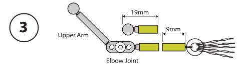
6. When the Epoxy Glue has completly set cut the Forearm to a length of 19mm and the Wrist to a length of 9mm.
