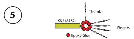
7. Equispace the fingers and create a thumb and glue them in place using Epoxy Glue. When the Glue has cured turn the hand/palm assembly over and glue on the other side.
